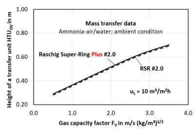
The efficiency of **Raschig Super-Ring® Plus #2** is practically the same as Raschig Super-Ring® #2
