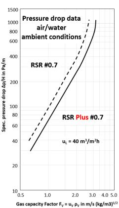
In the air/water simulator the pressure drop and capacity advantage is also proved for Raschig Super-Ring<sup>®</sup> Plus #0.7. A capacity advantage of 8 % and pressure drop reduction of min. 10 % was measured.
