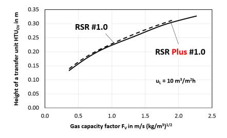
The efficiency of **Raschig Super-Ring® Plus #1** is practically the same as Raschig Super-Ring® #1
