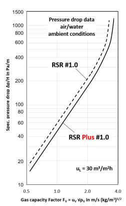
In the air/water simulator the pressure drop and capacity advantage is also proved for Raschig Super-Ring<sup>®</sup> Plus #1. A capacity advantage of 8 % and pressure drop reduction of 10 % was measured.
