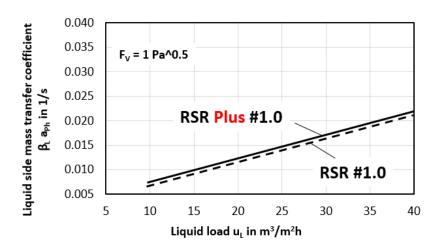
Absorption of NH3 from air in water in the gaseous phase
