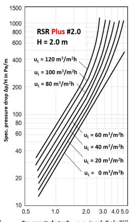
Gas capacity factor  $F_V = u_V \rho_V$  in m/s  $(kg/m^3)^{1/2}$
