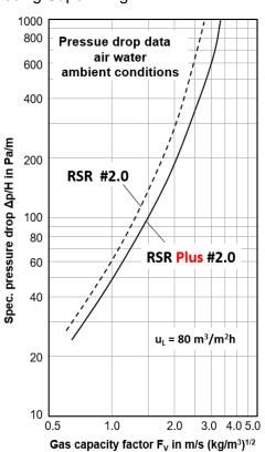
In the air/water simulator the pressure drop and capacity advantage of **Raschig Super-Ring® Plus #2** became obvious. The packing opens up the column cross section area by its special design which results in noticeable fluiddynamic benefits. A **capacity advantage of 8 %** and **pressure drop reduction of 10 %** was measured.
