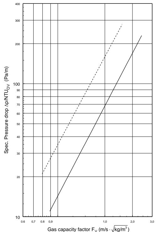
The graph shows the pressure drop related to 1-meter packed bed height as a function of the gas capacity factor  $F_V$ . The graph shows the differences in the dry and wet pressure drops between the 50 mm PALL Ring and the 50 mm RALU RING®.
