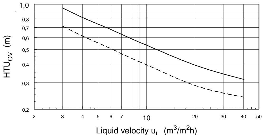
This graph shows the height necessary for the RALU-RING® in the gaseous phase of a transfer unit as a function of the irrigation density for the F factors:
