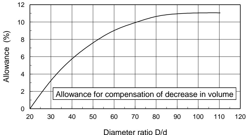
The values indicated in the tables for dumped packings are valid for a diameter ratio vessel: packing size of  $D : d = 20$ . Since the arrangement of the packings is less compact near the vessel wall than in the interior of the bed, the number of packings per cubic meter increases with the diameter ratio.
