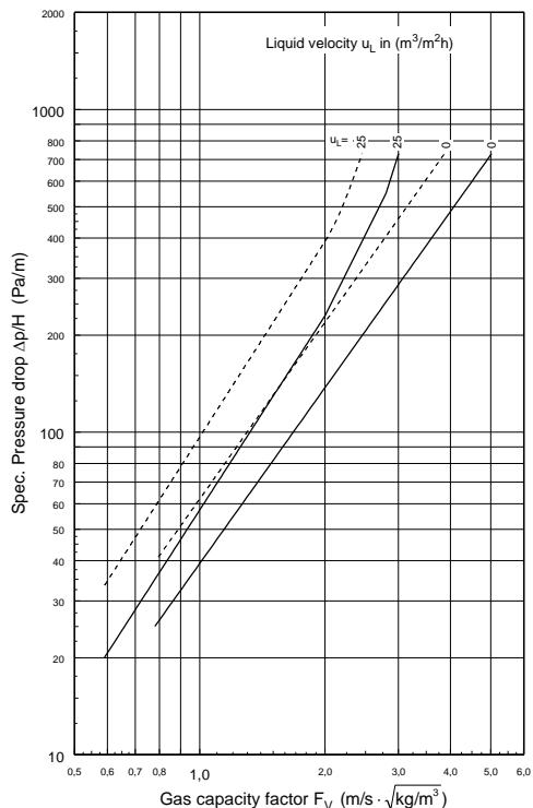
Specific pressure drop  $\Delta p/NTU_{OV}$  as a function of the gas capacity factor  $F_V$
